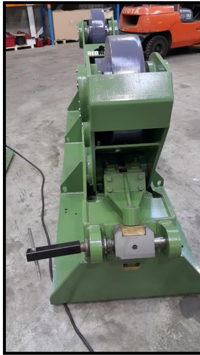
Idlers fitted with anti-creep feature
